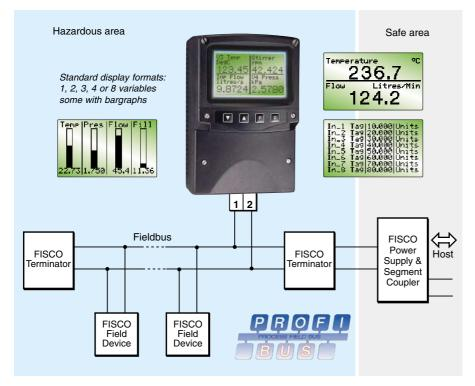
The BA484DF-P Fieldbus Display is an intrinsically safe instrument that can display up to eight fieldbus process variables. Eleven selectable standard screen formats contain one, two, three, four or eight variables, with units of measurement, tag descriptions and bargraphs on some screens.
